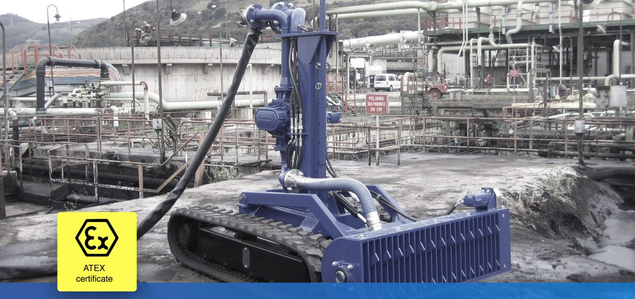
Hydraulically-operated submersible robot by remote control, specially designed for the extraction of sludge for PIT of any depth. The sludge extracted using the above mentioned methods must generally be processed to minimise the waste volume by dehydrating it and/or recovering the oil. To this end, we have mobile plants which allow performing these treatments on site, thereby avoiding the cost and transport risks associated with this waste type.
